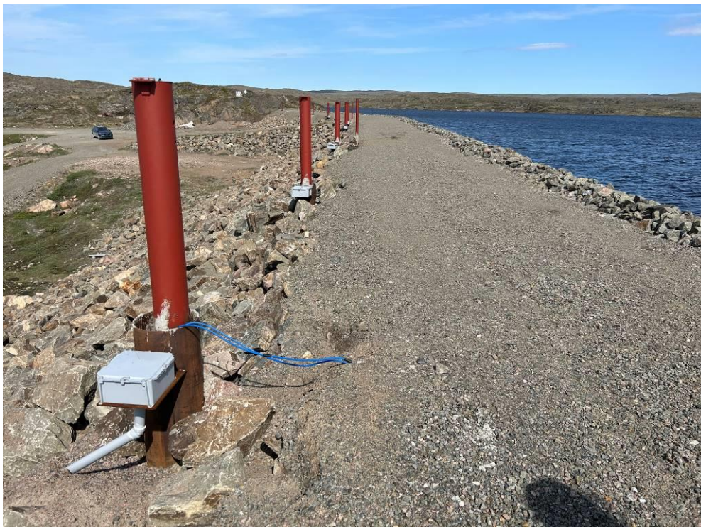
Photograph 12 – Typical temperature data logger installation.
