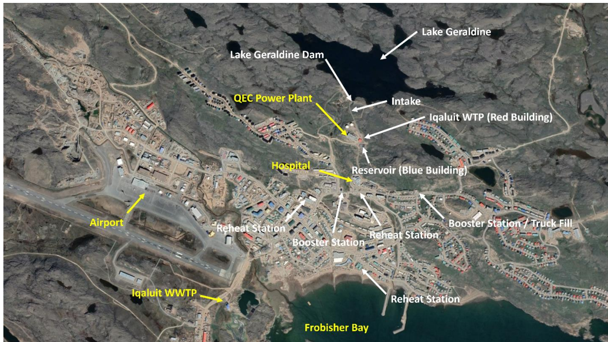
Figure 1-1: Water system components.
