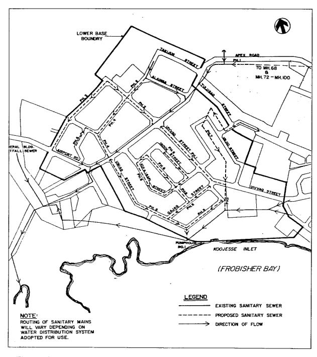
Figure 16 - RCPL Sanitary Expansion in Lower Base (after Figure 13, RCPL (1989))
