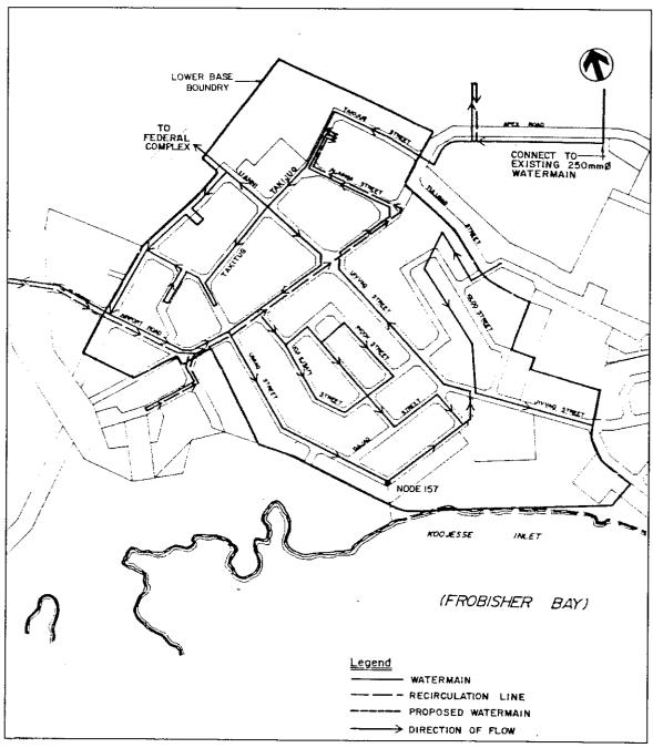
Figure 15 - RCPL Water Expansion in Lower Base (after Figure 7, RCPL (1989))
