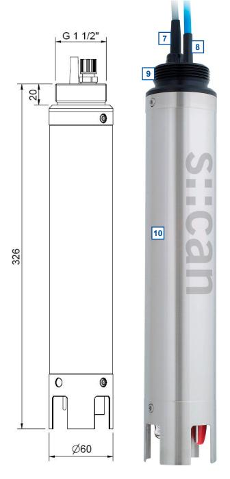
Dimensions of ammo::lyser / fluor::lyser in mm
