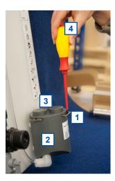
Remove the plug [3] from the flow cell [2]. To remove the plug insert a flat screw driver [4] into the small hole on the side of the flow cell and move the plug out by moving the screw driver downwards.
