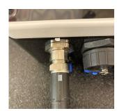
For initialisation on a D-315 con::cube the con::nect B-33-012 must be used. Connect the spectrometer to the con::nect via M12 plug and use a network cable to connect the con::nect to the con::cube. In addition the IP settings of D-315 and spectrometer have to be configured to the same address range (please refer to manual con::nect B-33-012).
