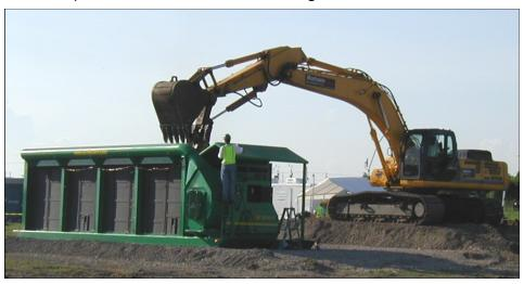
dles, or green branches such as palm fronds. While these are certainly ok to burn in the firebox, you want to add them to a hot fire so they dry out and ignite quickly. To keep the temperature up and to maintain the highest throughput of waste you should mix the very burnable wood with the less burnable materials throughout the course of the burning operation. The most common way to accomplish this is to stage a pile of the most burnable materials or what we call the "two pile system."
