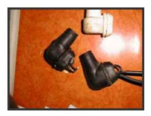
Figure 17: Assorted Mercury Freezer Switches for Disposal
