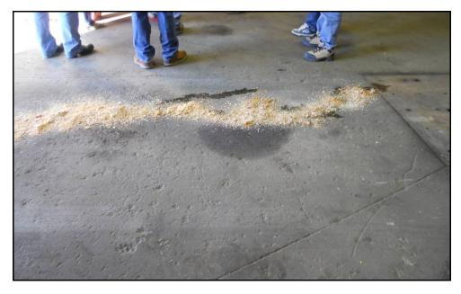
Figure 2: Absorbent Material place over Spilled Vehicle Fluids
