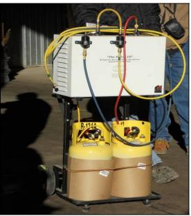
**Figure 9: Refrigerant Evacuation Unit**
