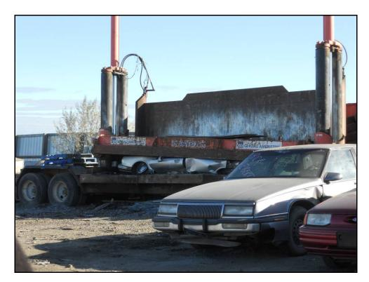
**Figure 5: Vehicle Crusher in Operation**
