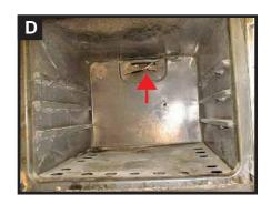
If you have determined that the gas oven capillary tubes and bulbs are mercury containing, the following procedure can be used to identify and remove the mercury gas safety valve control assembly.
