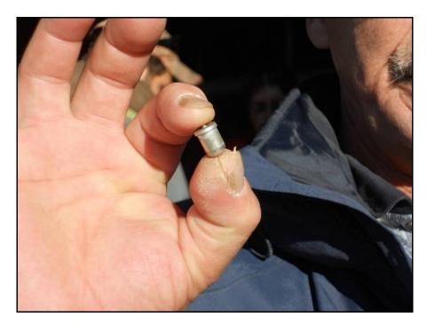
Figure 16: Mercury Pellet removed from Vehicle Convenience Light
