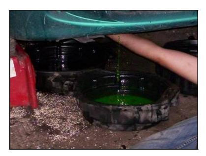
Figure 11: Using Drip Pans to Catch Draining Fluids
