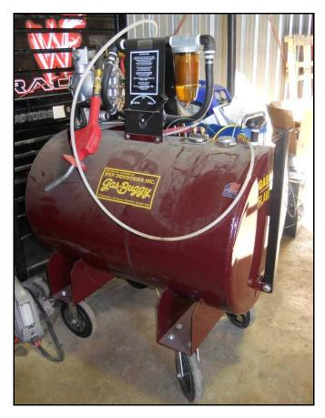
Figure 10: Example of Gasoline Collection System
