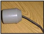
Sump pump float containing mercury.
