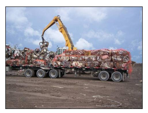
Figure 6: Example of "Logged" Metal
