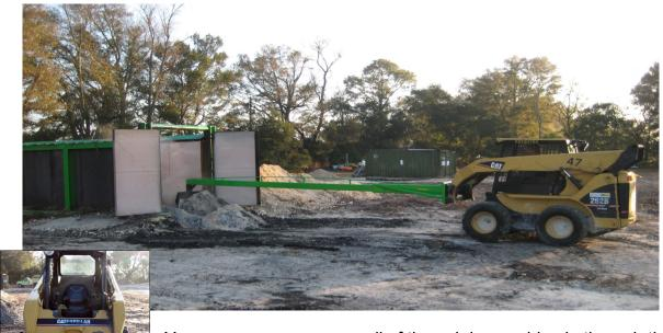
You can remove some or all of the ash by reaching in through the rear doors with the ash rake and dragging the ash out. Remember to use the appropriate breathing apparatus, and be cautious of the remaining hot embers. It is not required to remove all the ash if you are planning on a restart, generally just a
