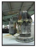
A mercury-free sump pump. Notice the metal guide and no attached wires.
