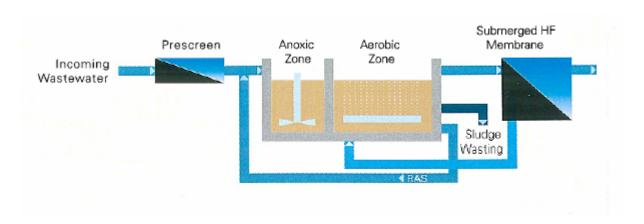
Figure 2. Immersed MBR configuration, including nitrogen removal steps.
