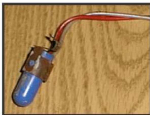
Figure 19: Washing Machine Mercury Switch
