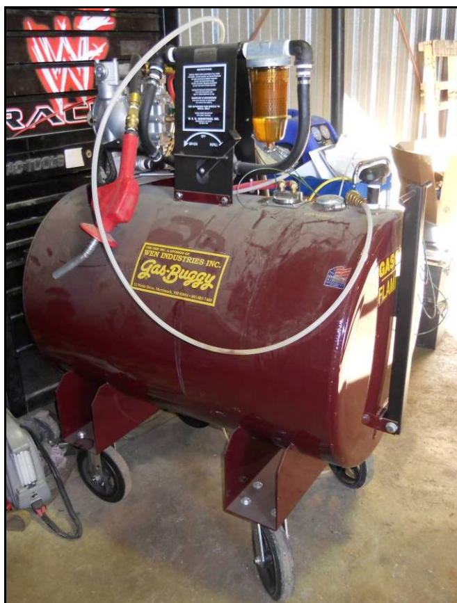
Figure 10: Example of Gasoline Collection System
