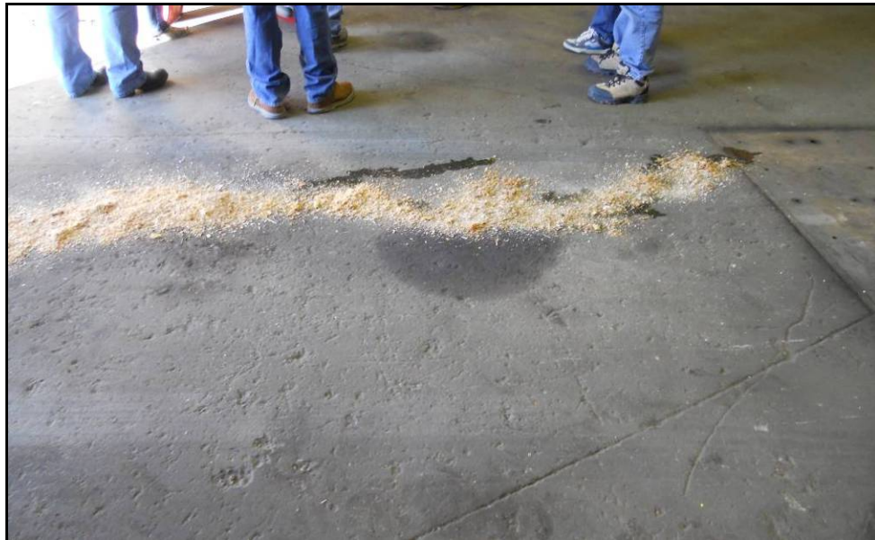
Figure 2: Absorbent Material place over Spilled Vehicle Fluids
