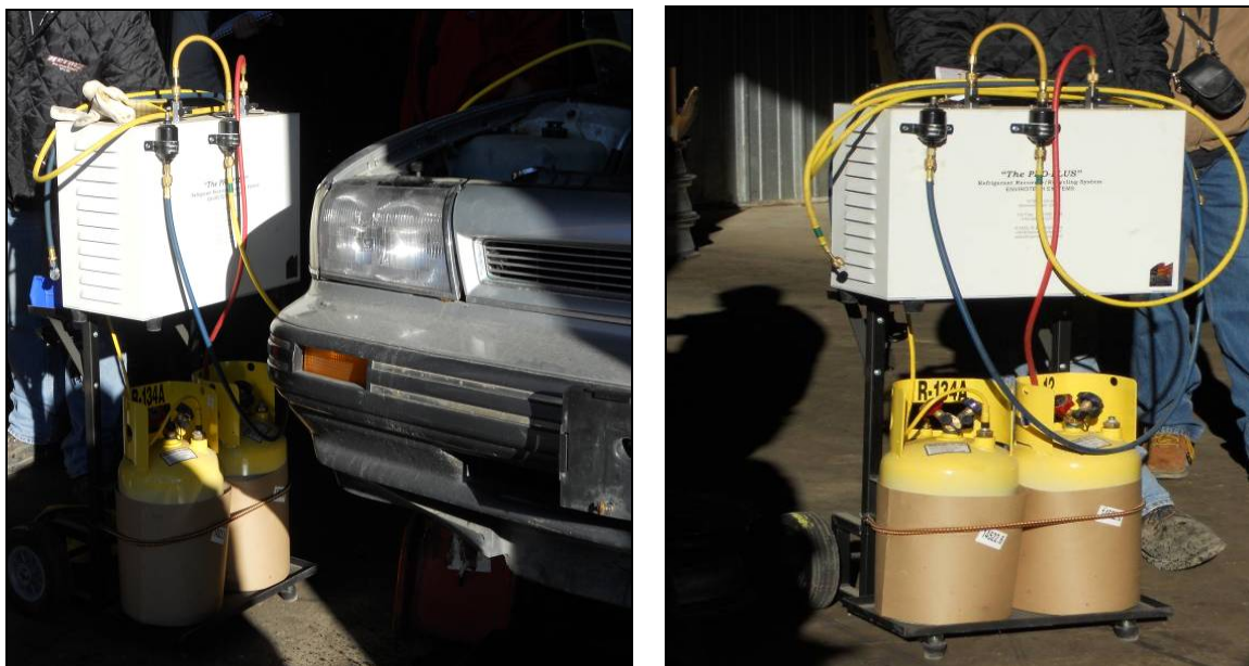
Figure 9: Refrigerant Evacuation Unit
