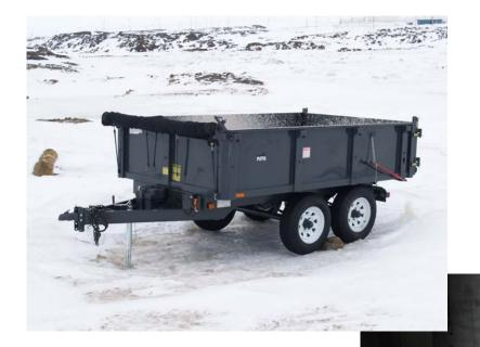
Sewage sludge transportation trailer – note rollout cover at front of trailer
