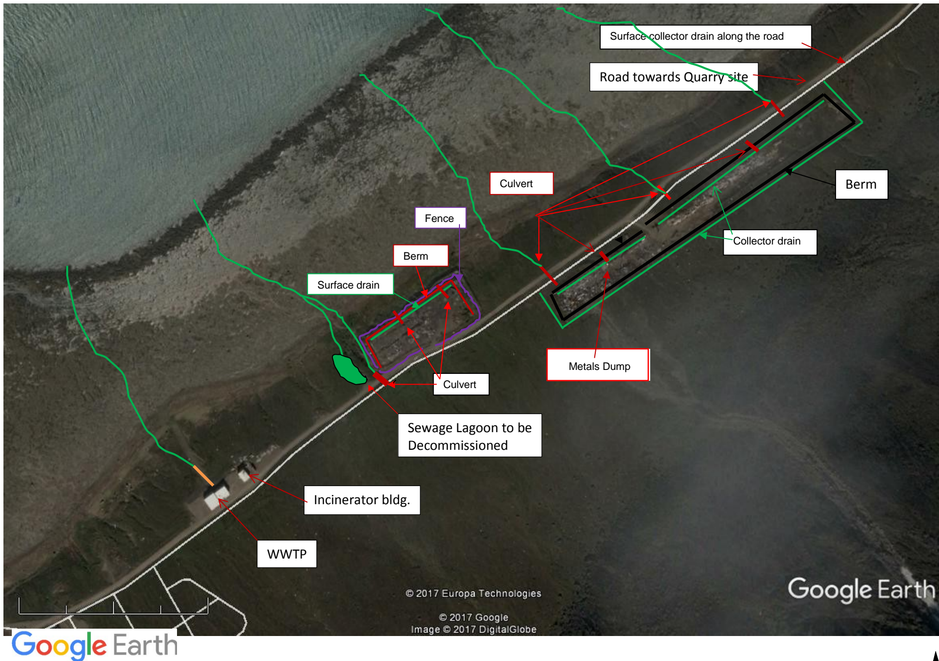
Aerial Photo of Pangnirtung Waste Facilities and Drainage network
