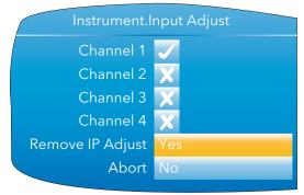
Figure 4.1.9e Channel adjustment removal
