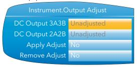
1A1B and 2A2B can be configured only as mA outputs.
