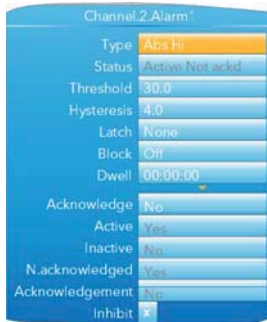
Figure 7.1a Channel 2, Alarm 1 set up
