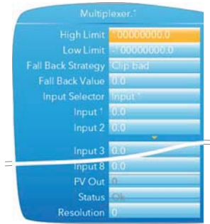
Figure 4.22 Multiplexer block configuration
