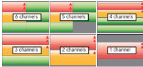
Figure 3.4.6b Alarm panel display layouts for trend groups with fewer than six channels
