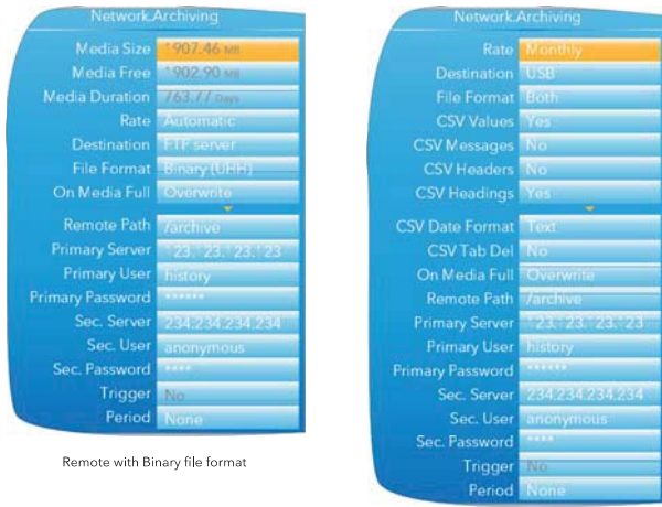
Figure 4.2.2a Unattended Archive configuration (typical settings)
