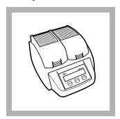
1. Set the DRB200 reactor power to on. Set the temperature to 100 °C.
