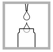
2. Add 1.3 mL of sample, 1.3 mL of Solution A and 1 Reagent B tablet in quick succession to a dry 20-mm reaction tube. Close the reaction tube
