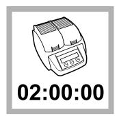
**8.** Keep the vial in the reactor for 2 hours.
