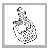
**6.** Insert the vial in the preheated DRB200 reactor. Close the lid.
