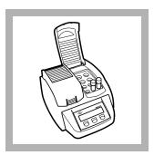
**3.** Insert the reaction tube in the preheated DRB200 reactor. Close the lid.
