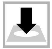
**16.** Insert the vial into the cell holder. DR 1900 only: Push **READ**. Results show in mg/L  $PO_4^{3-}$ .
