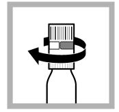
**4.** Turn the DosiCap Zip over the test vial so that the reagent side goes on the vial. Tighten the cap on the vial.
