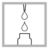
2. Use a pipet to add 0.5 mL of Solution B to the test vial. Immediately tighten the cap on the Solution B container.
