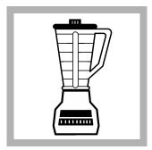
2. Measure 100 mL of sample in a blender. Blend for 30 seconds or until homogenized. If the sample does not have suspended solids, ignore this step.
