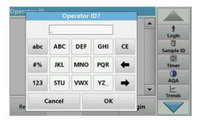
This display is used to enter letters, numbers and symbols as needed when programming the instrument. Unavailable options are disabled (grayed out). The icons on the right and left of the screen are described in Table 1
