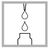
**3.** Use a pipet to add 0.4 mL of sample to the test vial.
