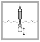
5. Field tests: Immerse the probe directly into the sample. Move the probe up and down to remove bubbles from the probe.
