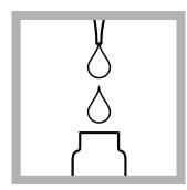
**12.** Use a pipet to add 0.2 mL of Solution D to the test vial.
