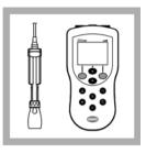
**2.** Connect the probe to the meter.
