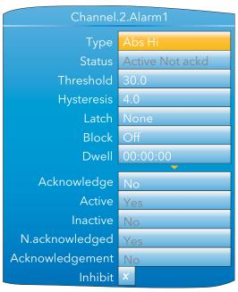
Figure 7.1a Channel 2, Alarm 1 set up
