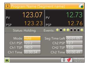
Figure 3.4.9b two channel program in Hold mode
