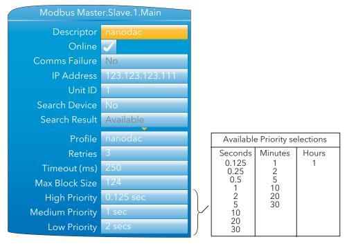
Figure 4.9.1 Modbus Master Slave 1 configuration (Slave 2 similar)
