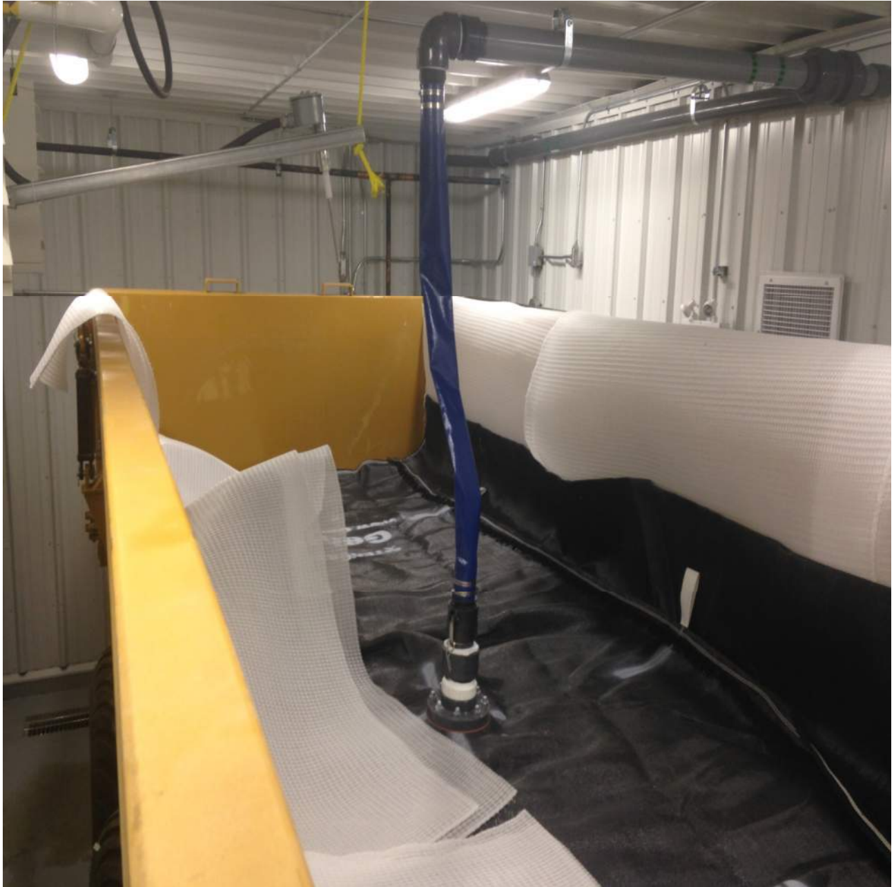
Figure 8: Geo-tube in the Trailer Ready to Receive Sludge
