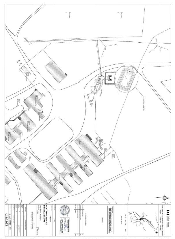
Figure 5. New Alert Landfarm Design at ALT-10 (Day Tank Fuel Farm) (Sept. 2013).
