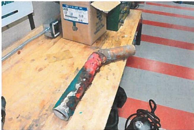
Figure 3 – Cause of the glycol spill was due to corrosion of the heat recovery pipeline.
