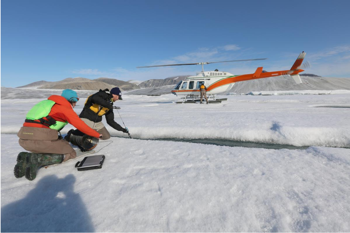
Profiling of ocean salinity and temperature through a crack on the Milne Ice Shelf.
