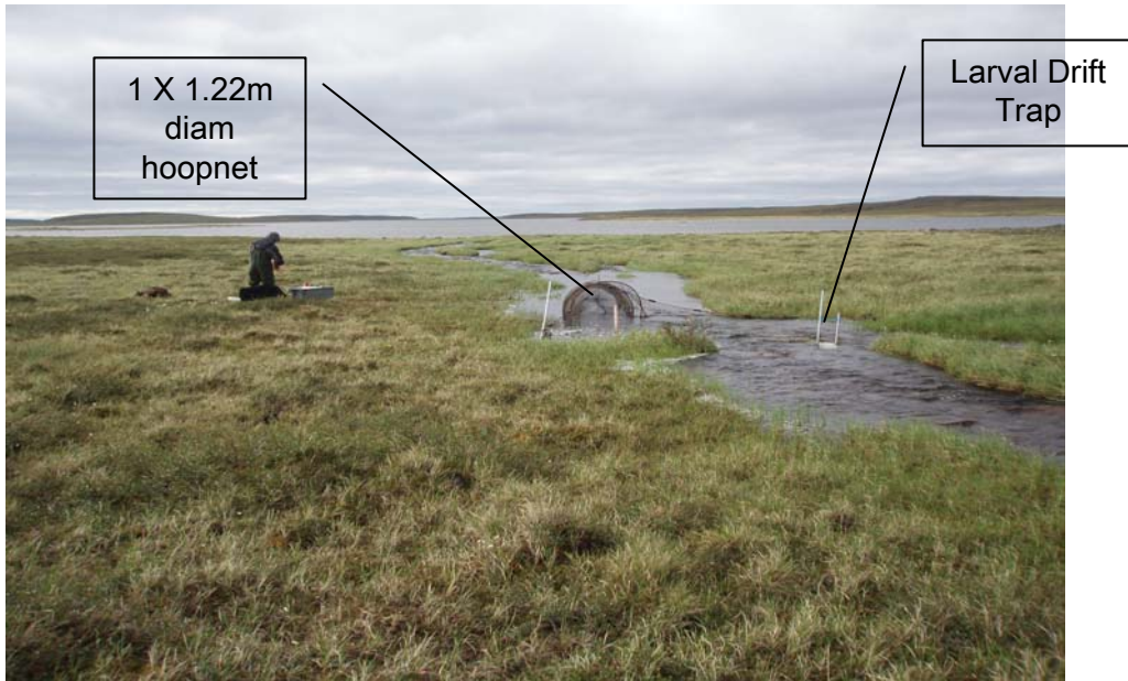
July 17/05 Hoopnet collecting fish migrating downstream and drift trap in foreground at B05
