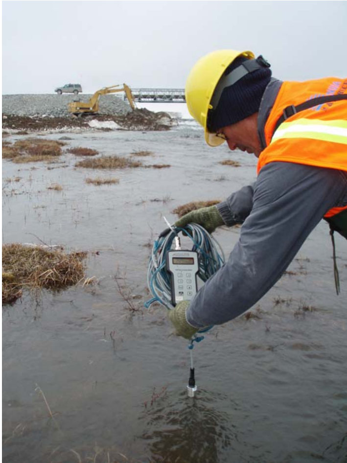
Photo 5. R02 – Turbidity monitoring downstream during stockpile removal (D/S S side) (16Jun07)
