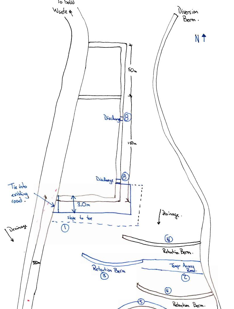
Discharge / cip rap. fill gradual slope, and armour with sip rap - 150 mm depth min install fill gradual slope and armour with rip rap - 150 mm depth my ربه رط 17-100 - 150mm Invert of culvert
