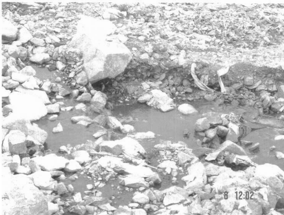
Figure 5. Effluent flow which is continuously discharged from the Hamlet of Baker Lake sewage lagoon.
