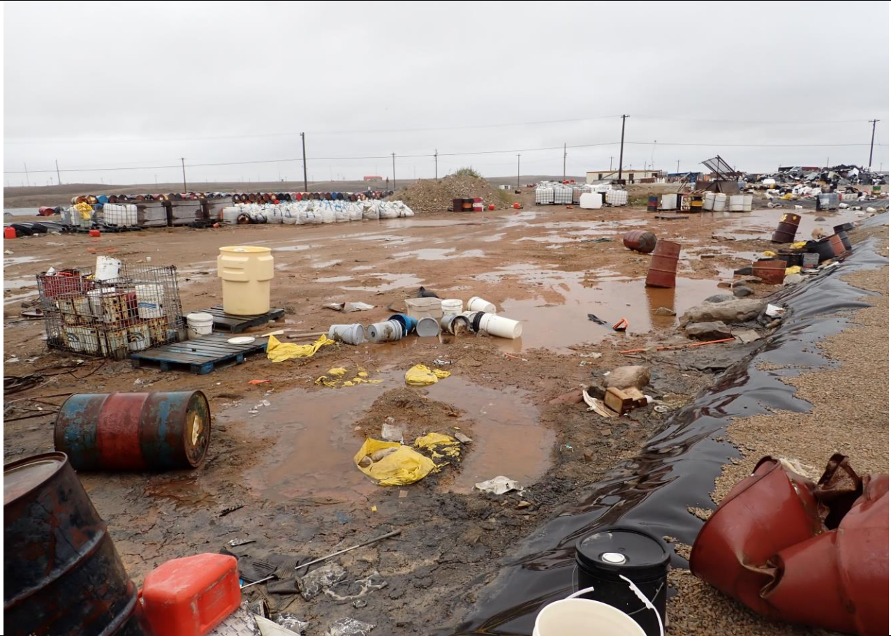
Description: under utilized hazardous water secondary containment.
