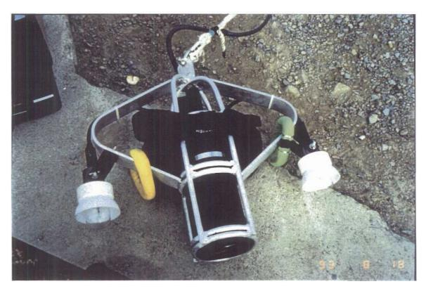
Photograph 2.6: Drop camera used to help identify targets located by side scan sonar.
