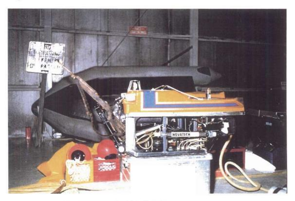
Photograph 2.4: Remote operated vehicle (ROV) equipped with video and sectorscan sonar. The object in the manipulator arm was retrieved from the bottom of Cambridge Bay.
