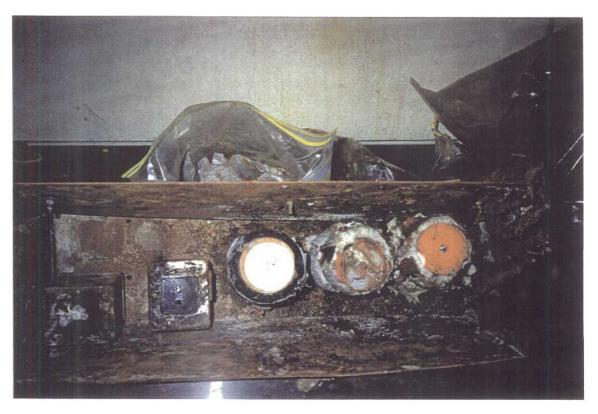
Photograph 3.17: Inside of a signal delay filter showing corrosion; two of four rectangular transformers and three copper coils.
