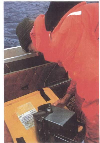
Photograph 2.8: Eckman grab, also used for sampling marine sediments.
