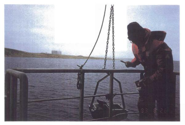
Photograph 2.7: Van Veen grab used for sampling marine sediment from the deck of the J.P. Tully, August 1993.
