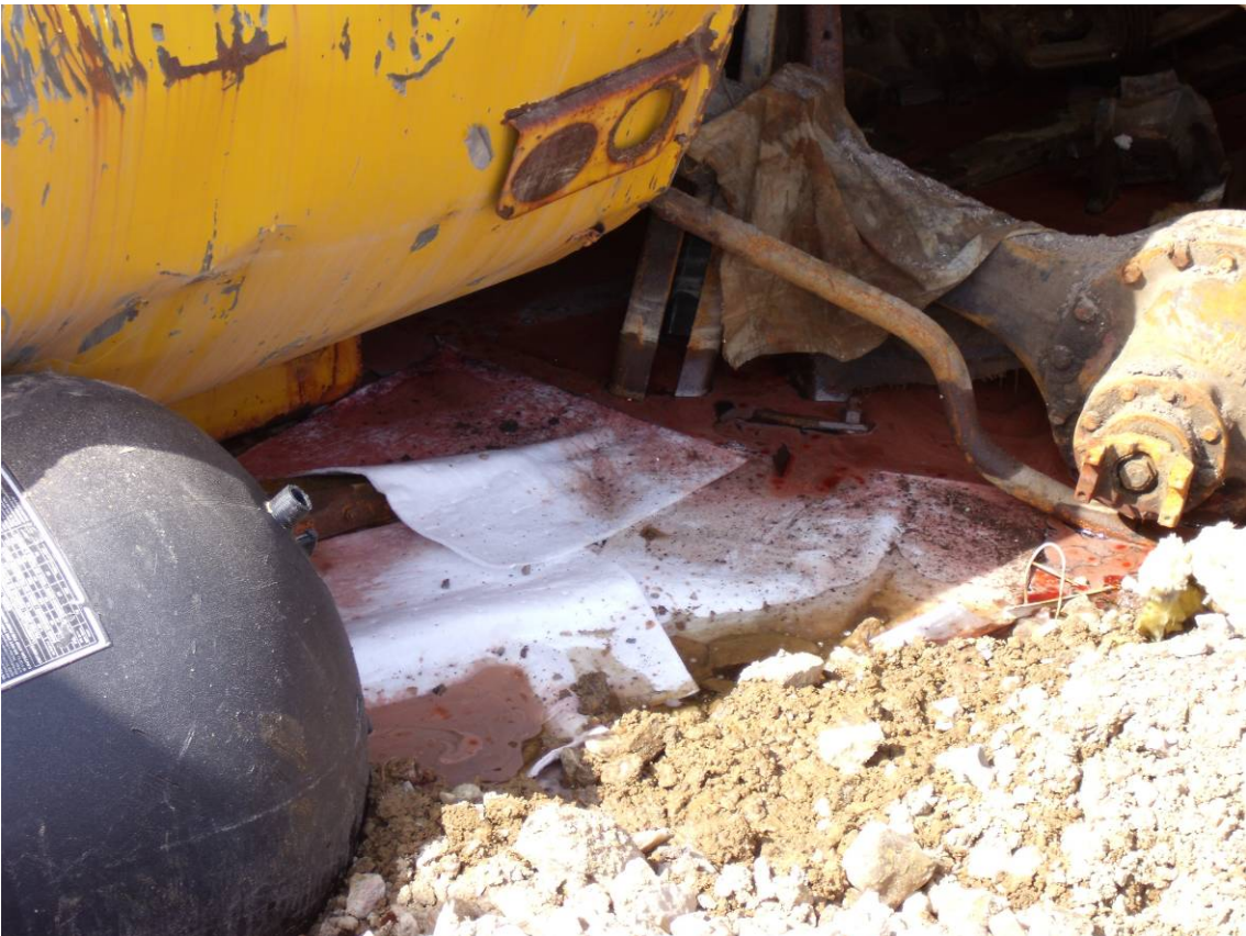
Photograph 16: Possible transmission fluid leaking from vehicle.
