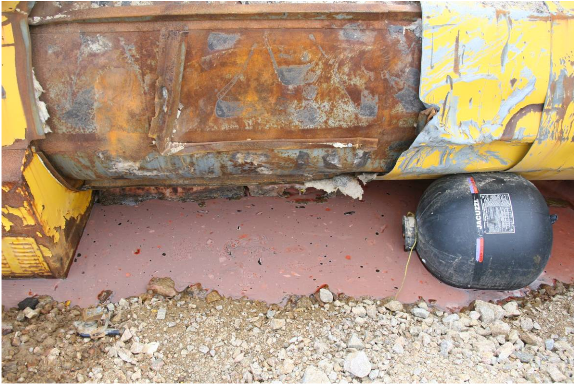
Photograph 15: Possible transmission fluid leaking from vehicle.
