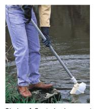
Any dedicated sampling equipment such as sampling poles (see photo on left for an example) are to be cleaned with soap and water after each sampling location to prevent cross-contamination. Other than the disposable gloves, a sampling pole to reach more difficult locations, and potentially polyethylene tubing and foot valves for groundwater sampling, no other sampling equipment is foreseen.
