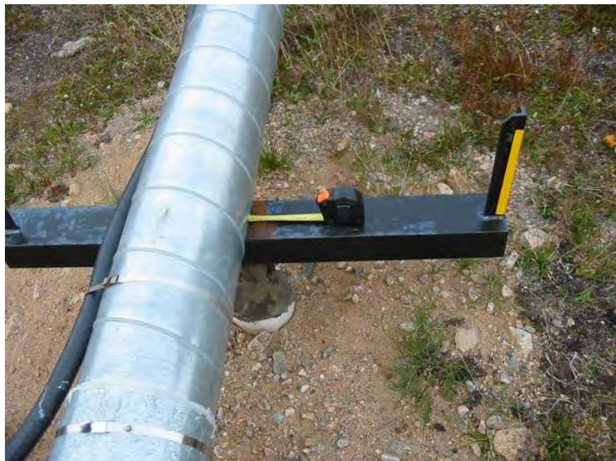
Photograph 16: Lateral displacement of pipeline on uphill leg of expansion loop.
