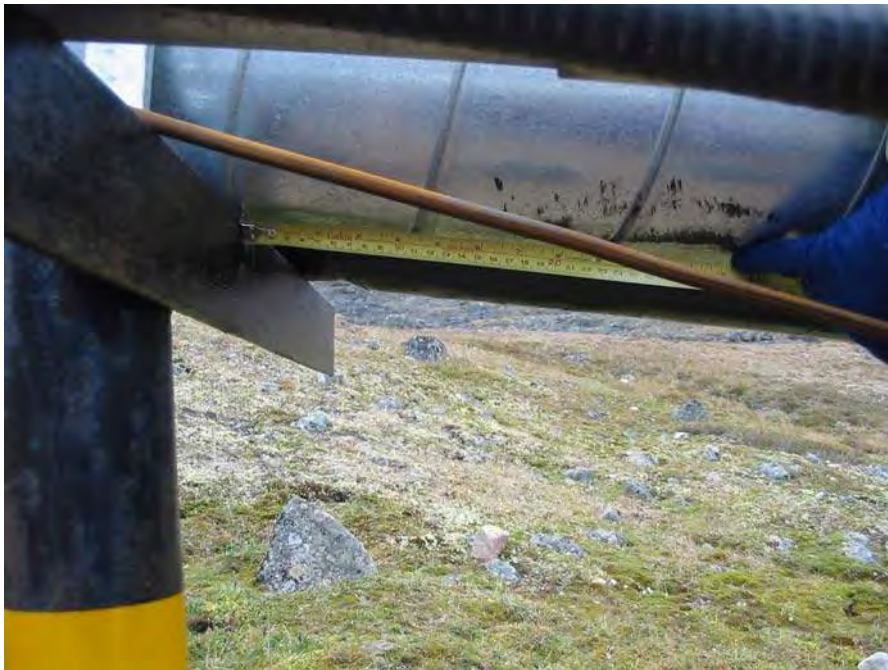
Photograph 20: Approximately 235 metres downhill of expansion loop, displacement of approximately 15 inches.
