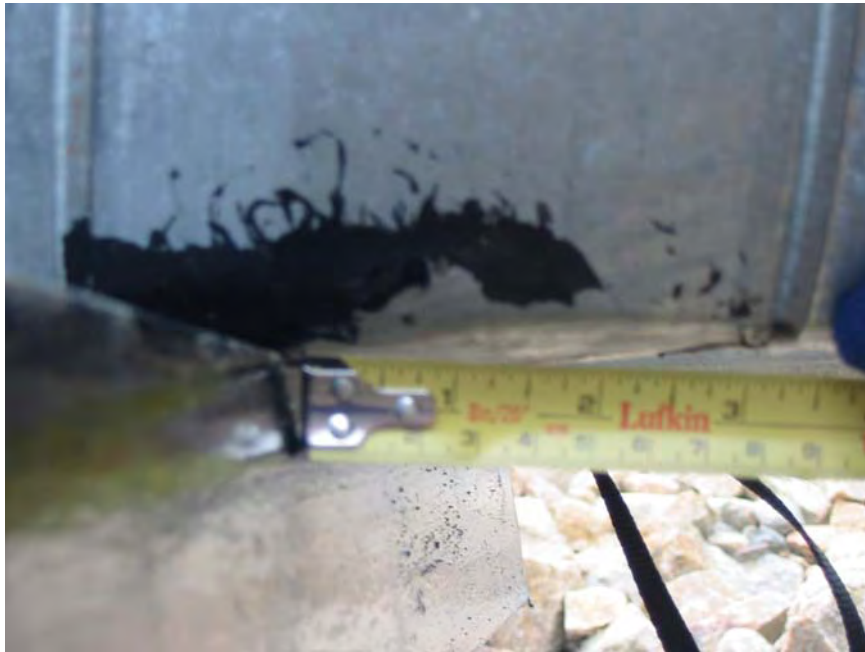
Photograph 29: Approximately 15 metres downhill of road crossing displacement of 3 inches.
