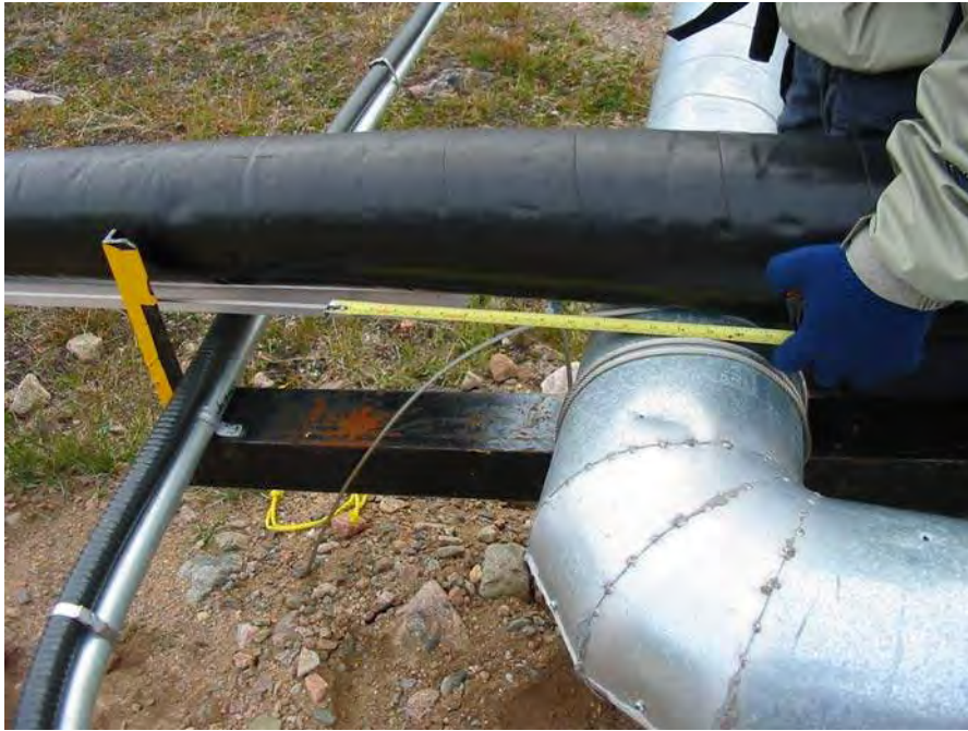
Photograph 17: Lateral displacement of pipeline on downhill leg of expansion loop.
