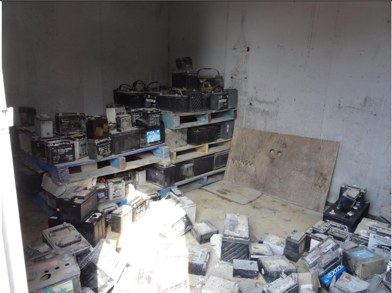
Description: Battery Storage Inside Shed with No Secondary Containment
