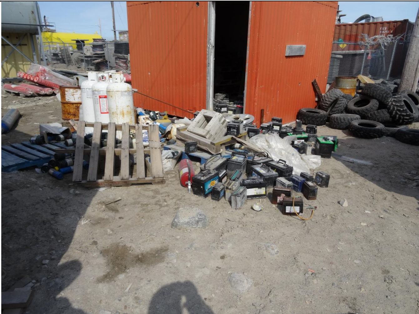
Description: Battery Storage Outside Shed on bear ground with No Secondary Containment
