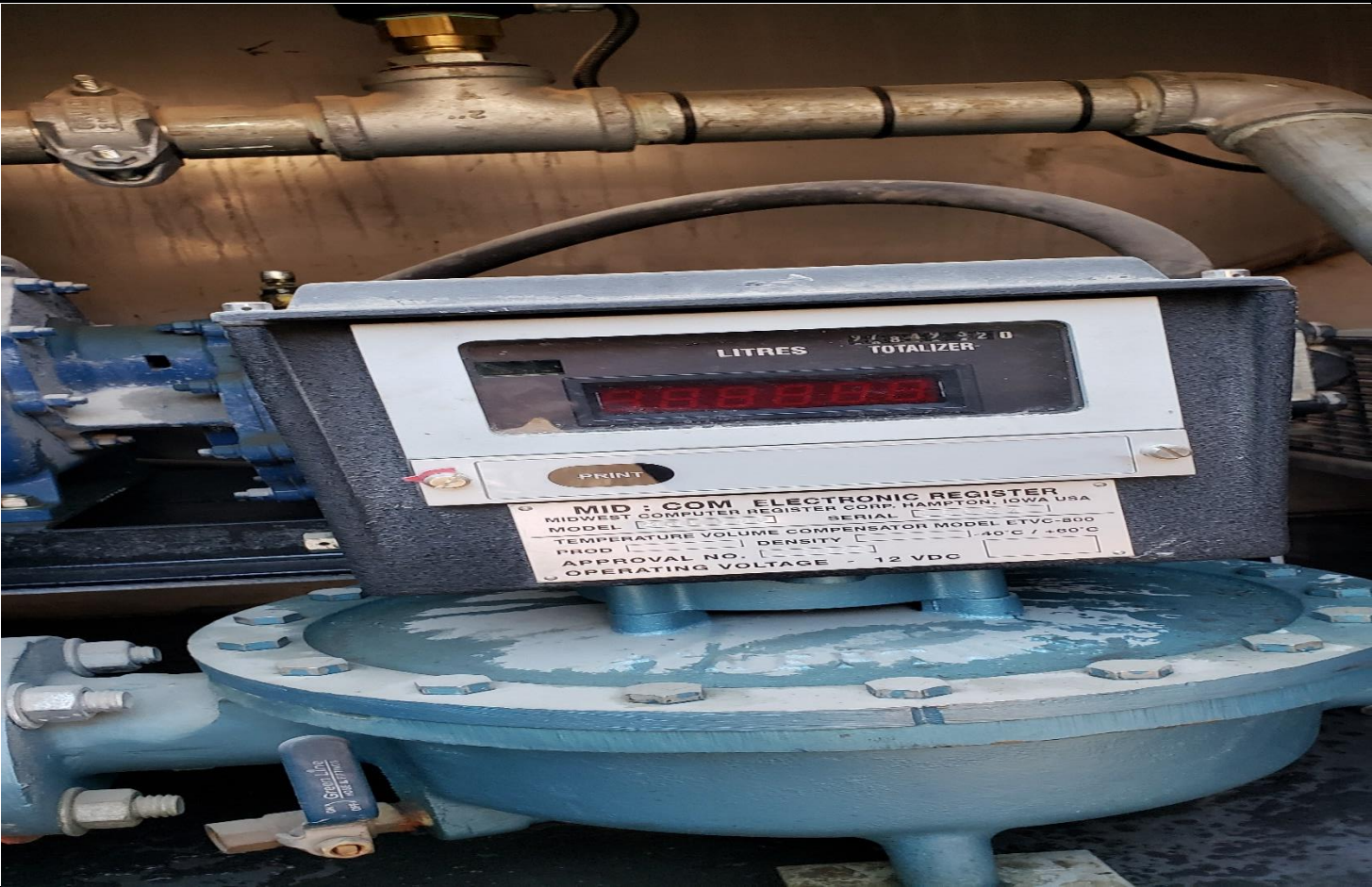
Description: Water Meter on the Water Delivery Truck.. Totalizer reads
