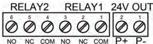
Figure 12. Relay & 24 V Output Connections
