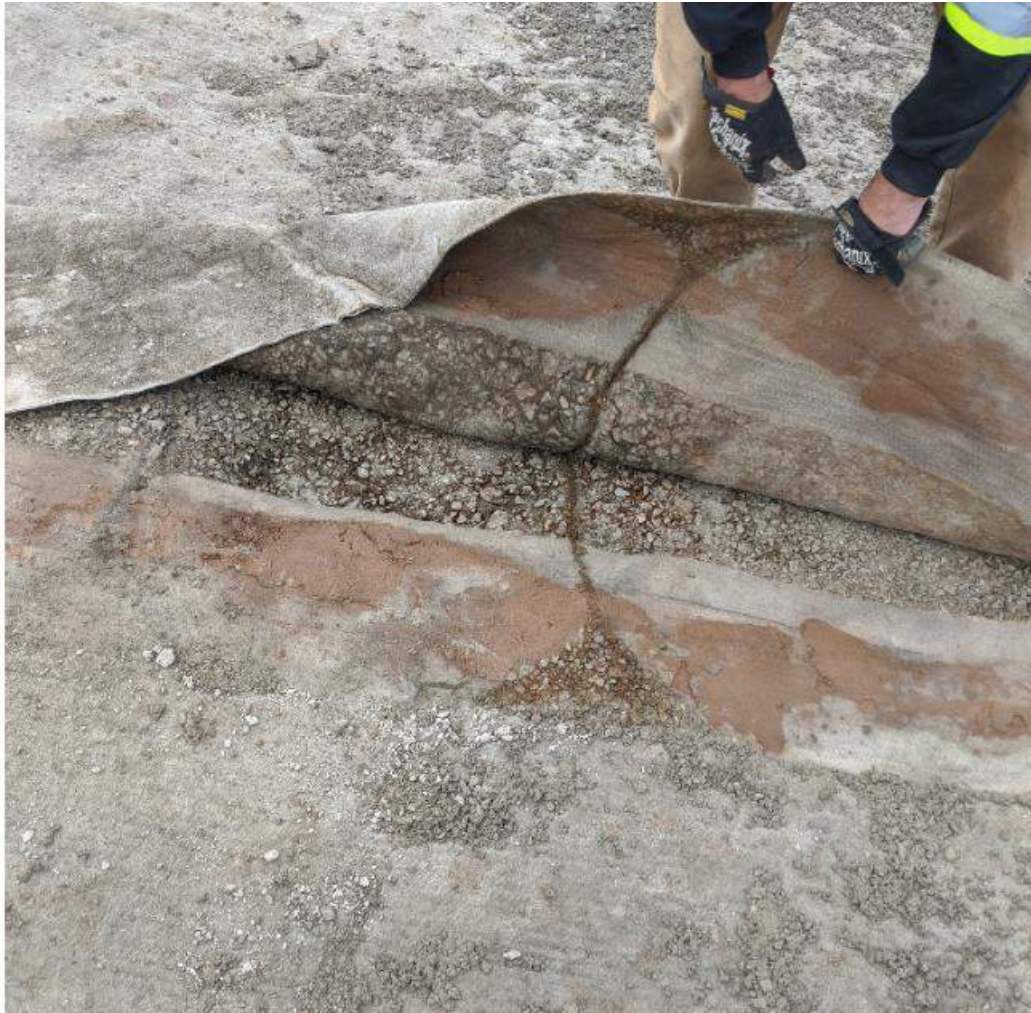
Photograph #1: Evidence of water travelling through a seam. The edge of the seam is held open by gravel.
