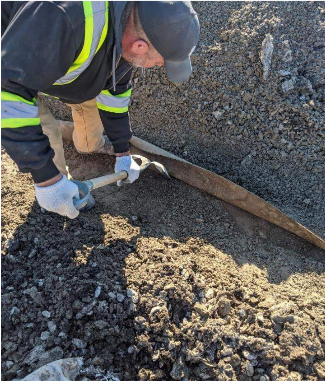
Photograph #1: Gravel in the northernmost east-west seam. Full penetration through the seam.
