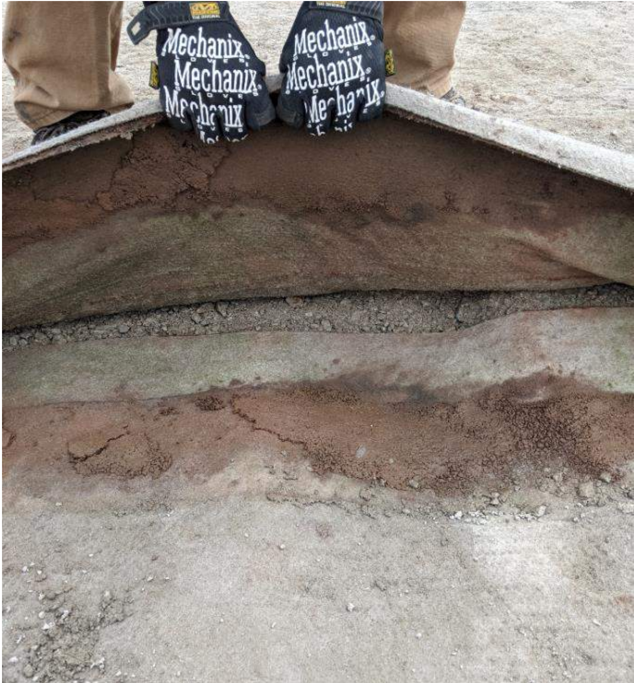
Photograph #4: The seam that was exposed was opened to examine the overlap and bentonite. The bentonite missing on the bottom flap is present on the top flap. It appears that a continuous strip of bentonite is formed.
