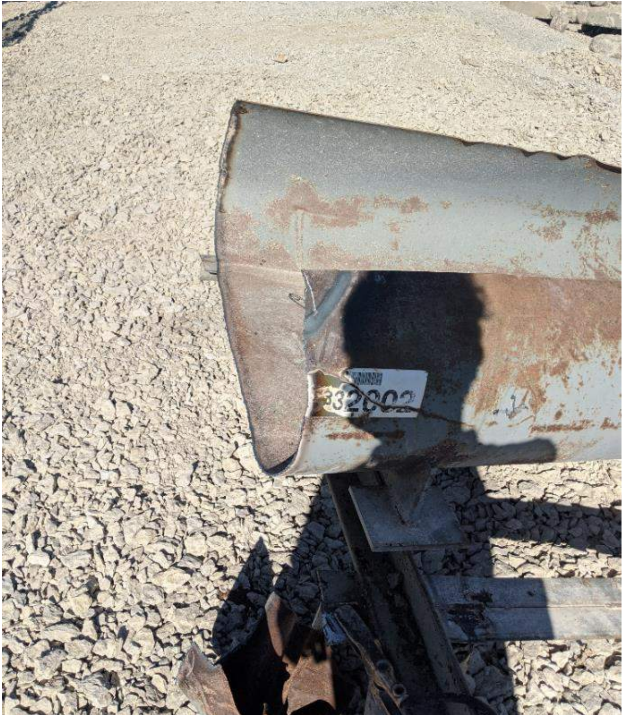
Photograph #2: The crumpled metal at the front of the chute at the north discharge station was cut off, leaving a straight edge.
