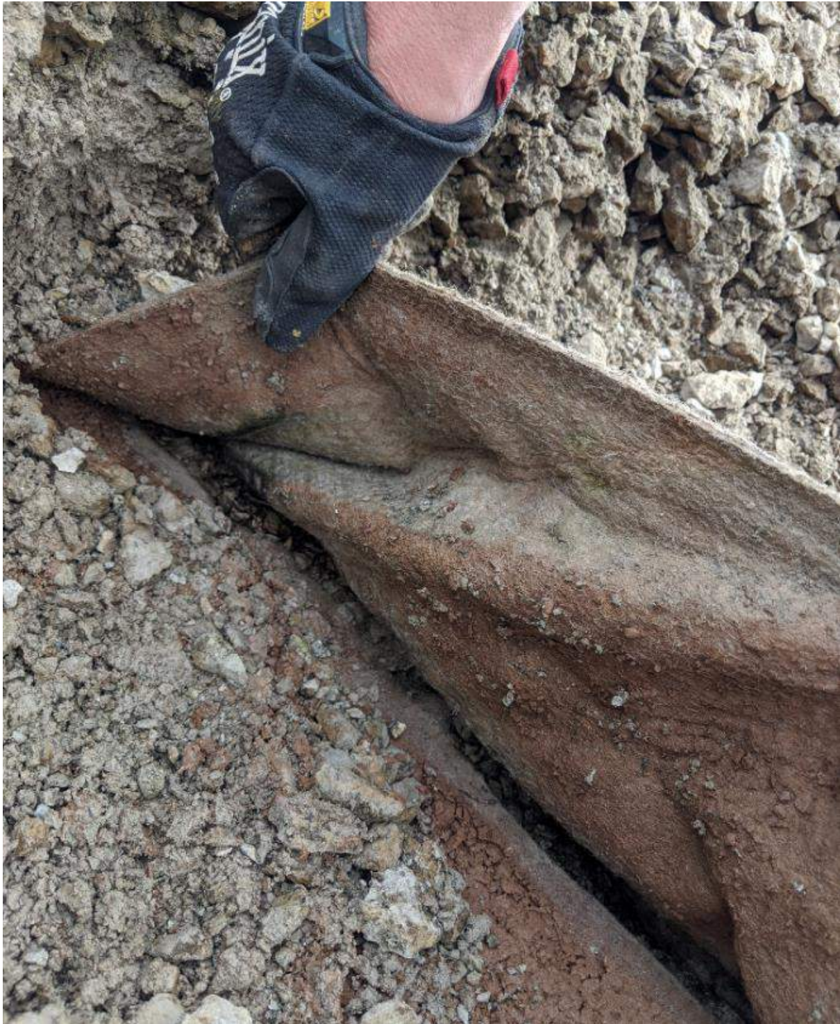
Photograph #2: Staining pattern within the seam. Note the lack of staining running along the center fold, suggesting that no bentonite was ever present in this fold, which was tightly closed and weighed down with aggregates. This fold is the one pointed to with the shovel in photograph 1.
