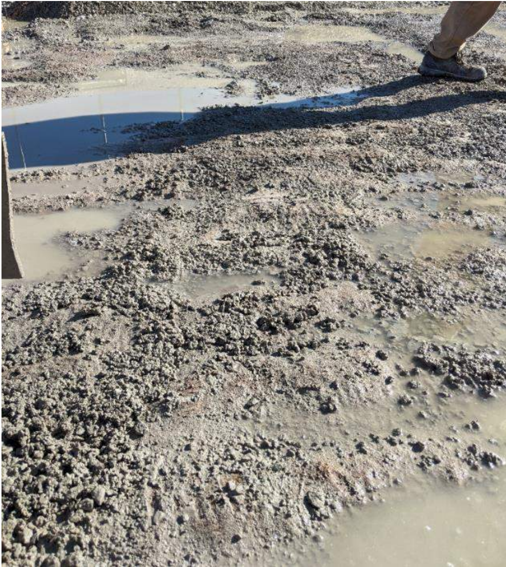
Photograph #1: Track patterns in liner (in foreground). The patterns are difficult to capture in a photo, but should be more visible once the water has dried up and the sand can be brushed away.
