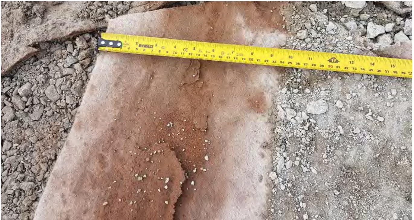
Photo 1: Evidence of overlap and bentonite at GCL seam at Area 1.
