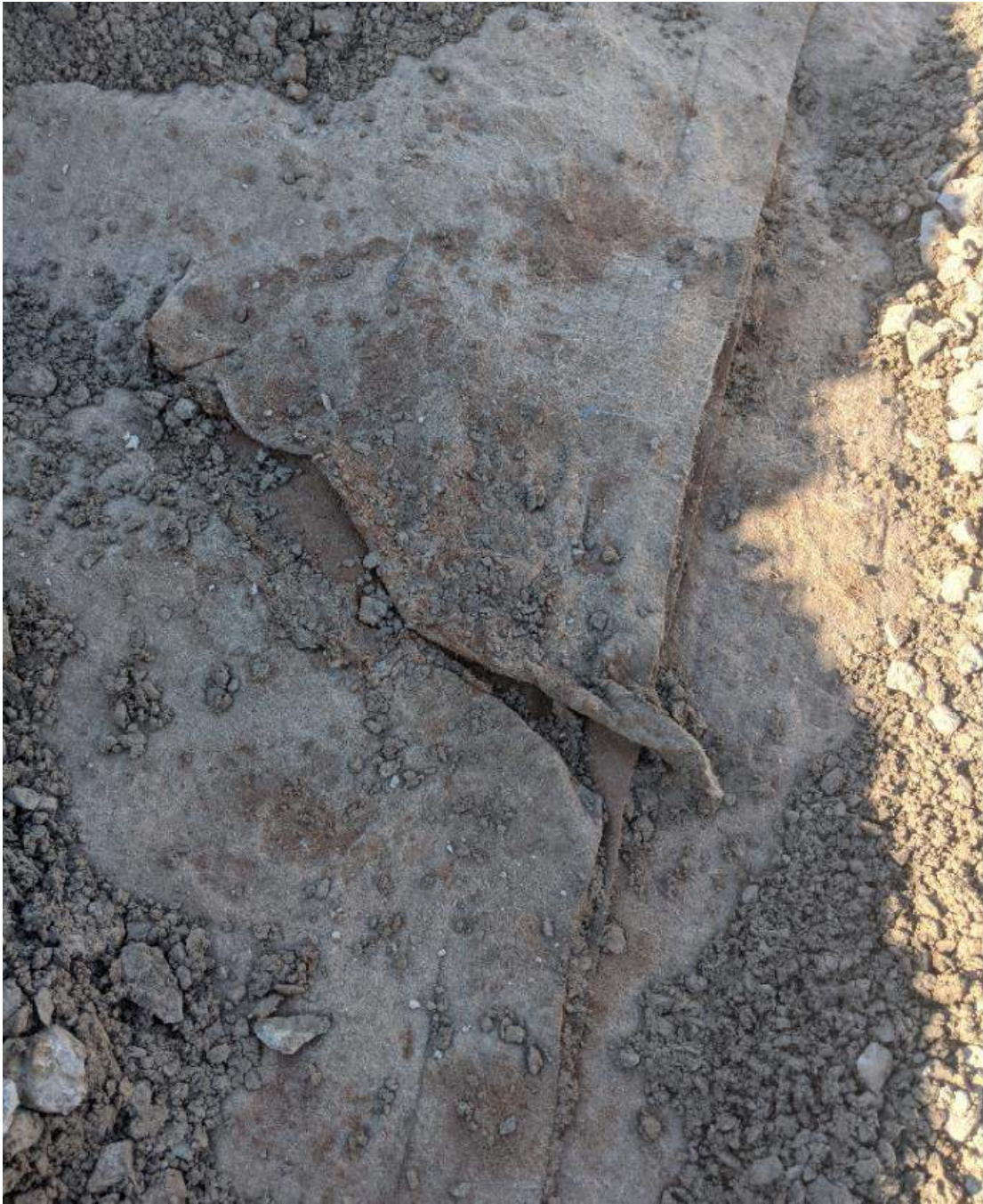
Photograph #1: Large tear found in one of the seams.
