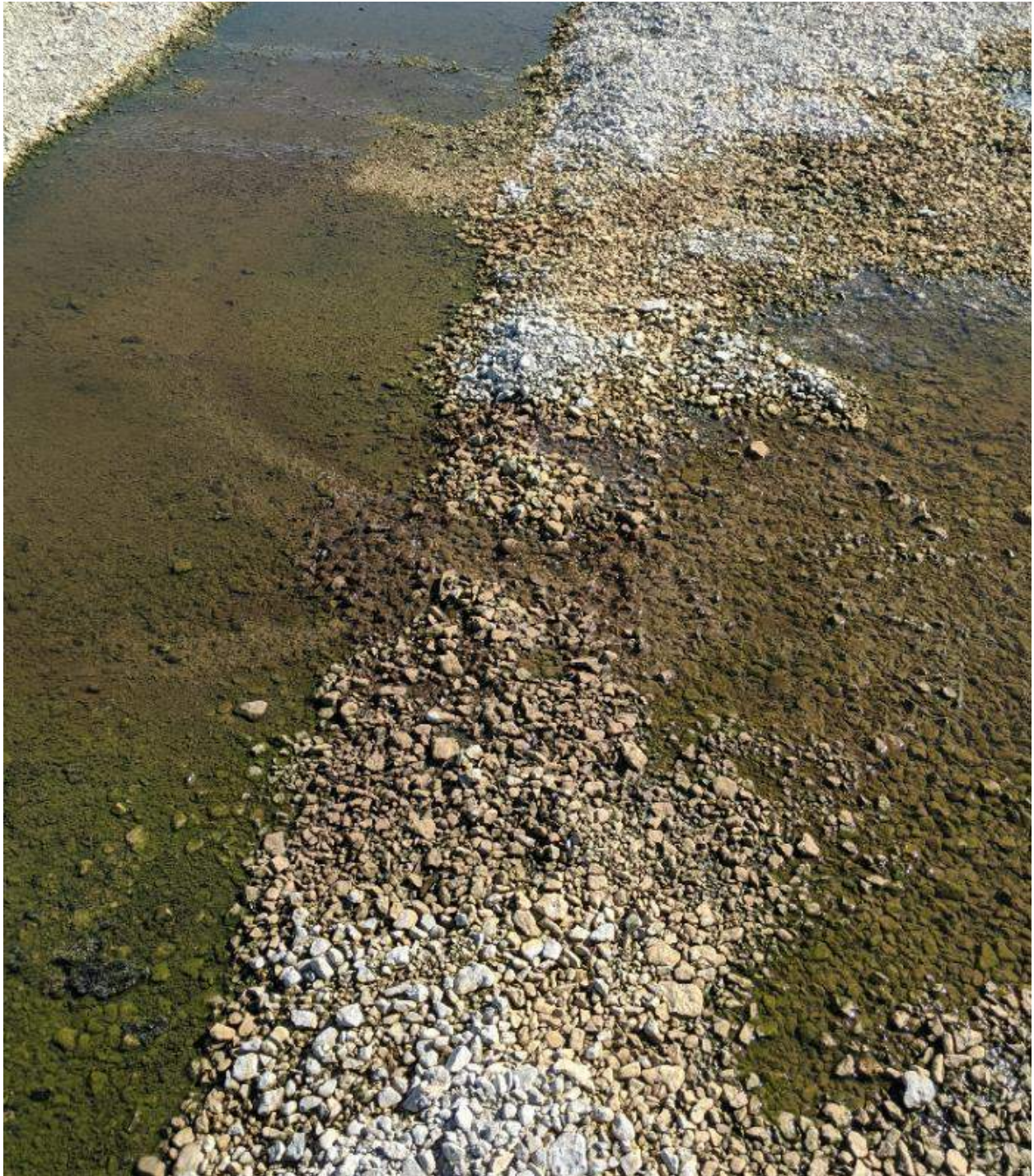
Photograph #2: The leak is beginning to recede significantly in area. The orange discolored region represents the area formerly covered by flowing water.
