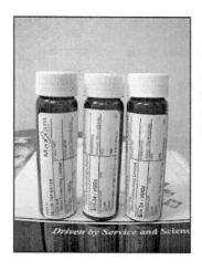
VOC Vials – These are three 40mL brown amber vials with white powdered preservative (Sodium Thiosulphate). All three vials must be filled with NO HEADSPACE; the vial must be filled to just overflowing. Fill slowly to half way point; swirl to ensure preservative is dissolved. Fill all the way to the top so the sample is just overflowing.
