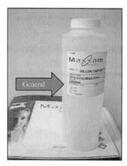
General Bottle – This bottle will also be a 500mL plastic bottle with no preservative. This container will be used for Alkalinity, Chloride, Conductivity, Hardness, Dissolved Calcium, Dissolved Magnesium, Nitrate, Nitrite, pH, and Sulphate.
