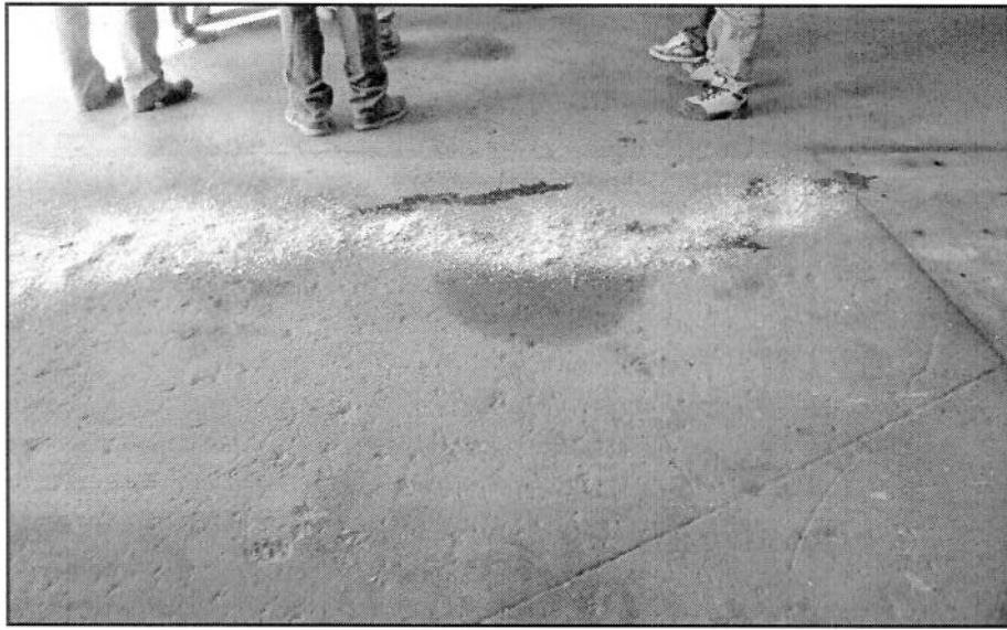
Figure 6. Absorbent Material place over Spilled Vehicle Fluids
