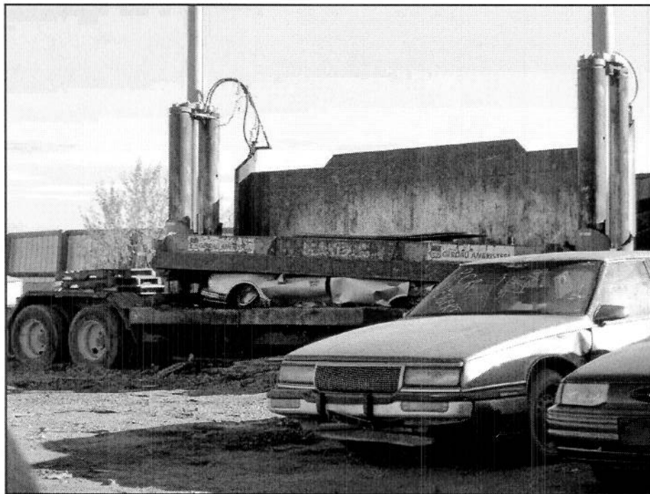
Figure 9. Vehicle Crusher in Operation
