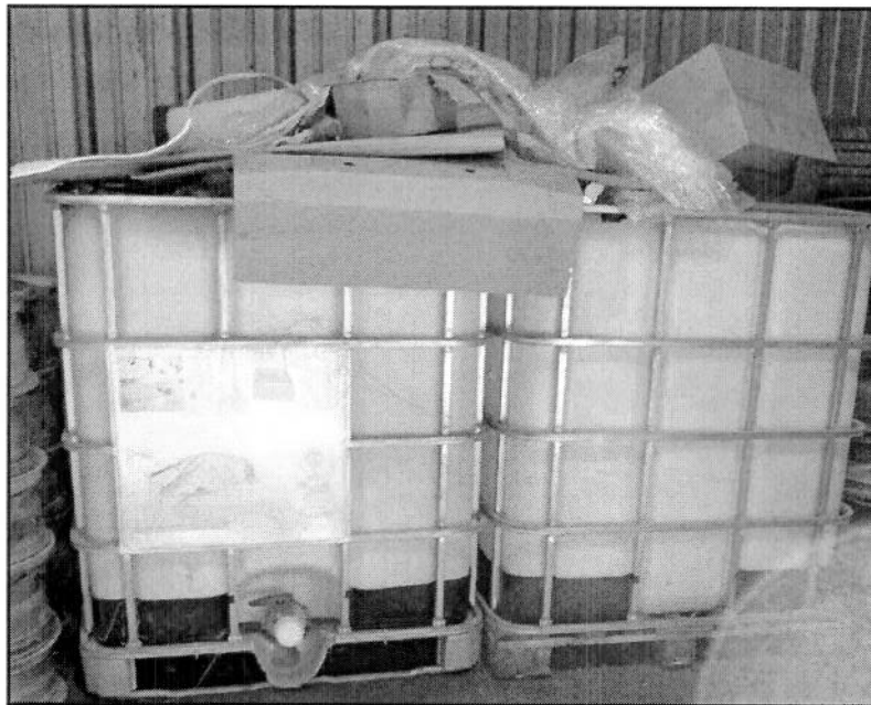
Figure 8. Example of Plastic Totes Used for Collection of Vehicle Fluids - Not Used for Gasoline
