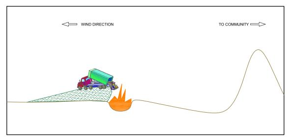
WASTE IS BURNED IN AN OPEN PILE OR WITHIN A BURN PIT. BURNING IN BURN PIT SHOULD TAKE PLACE WHEN THE WIND IS NOT BLOWING TOWARDS THE COMMUNITY.
