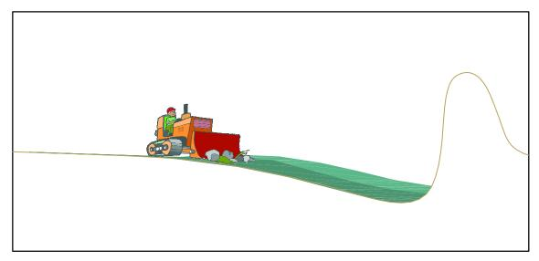
WASTE IS SPREAD OVER A SMALL AREA AND COMPACTED BY MAKING SEVERAL PASSES WITH THE EQUIPMENT. LAYERS SHOULD BE 250mm TO 300mm (10 TO 12 inches) FOR OPTIMAL WASTE COMPACTION. 50mm TO 100mm (2 TO 4 inches) OF COVER SOIL IS ADDED WHEN AN AREA (cellular layer) HAS BEEN FILLED.
