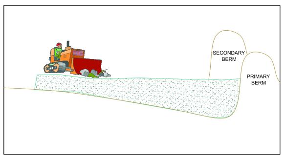
TO EXTEND SITE LIFE BEYOND THE HEIGHT OF THE INITIAL BERM ANOTHER BERM CAN BE CONSTRUCTED AND FILLING CAN CONTINUE.
