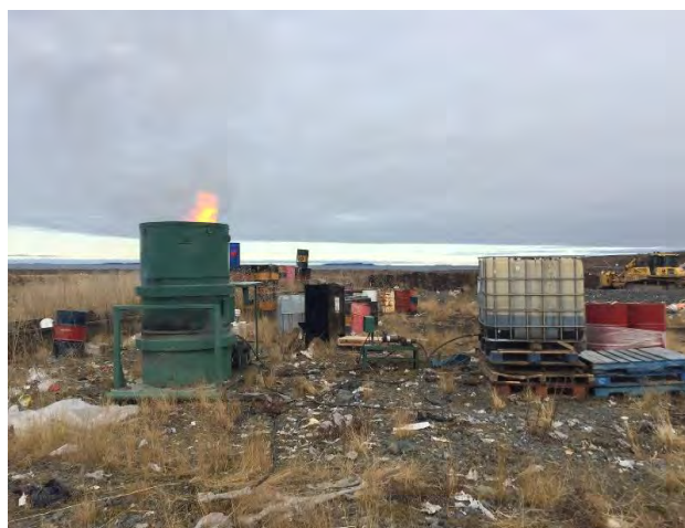
Waste oil burn incinerator
