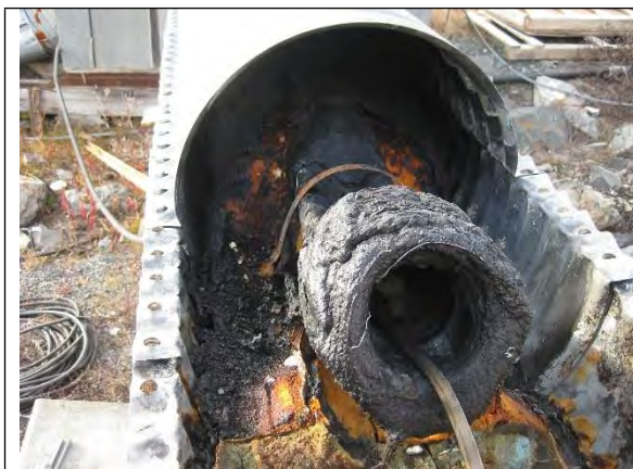
Photo 1: Burned tee to old pumphouse.
