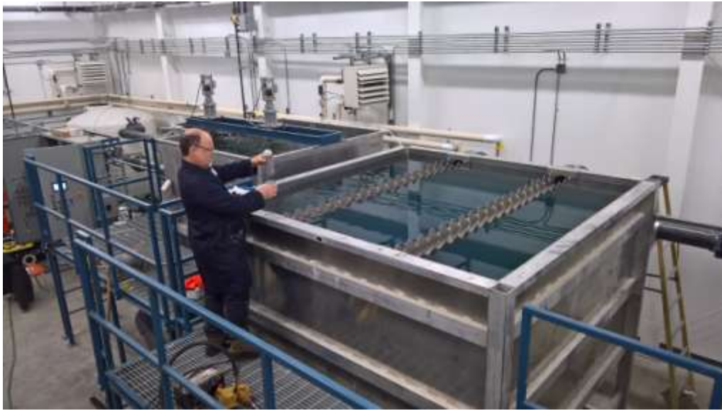
Fig. 6: Clarifier system for removing turbidity
