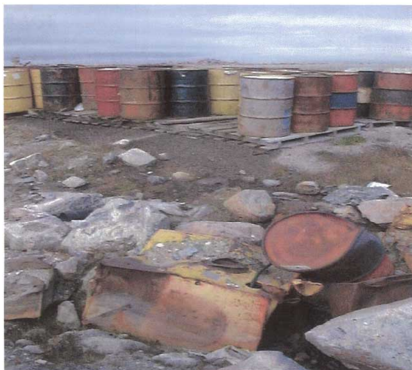
figure 6. Hydrocarbon contamination at the waste oil storage site; 2001/08/29.
