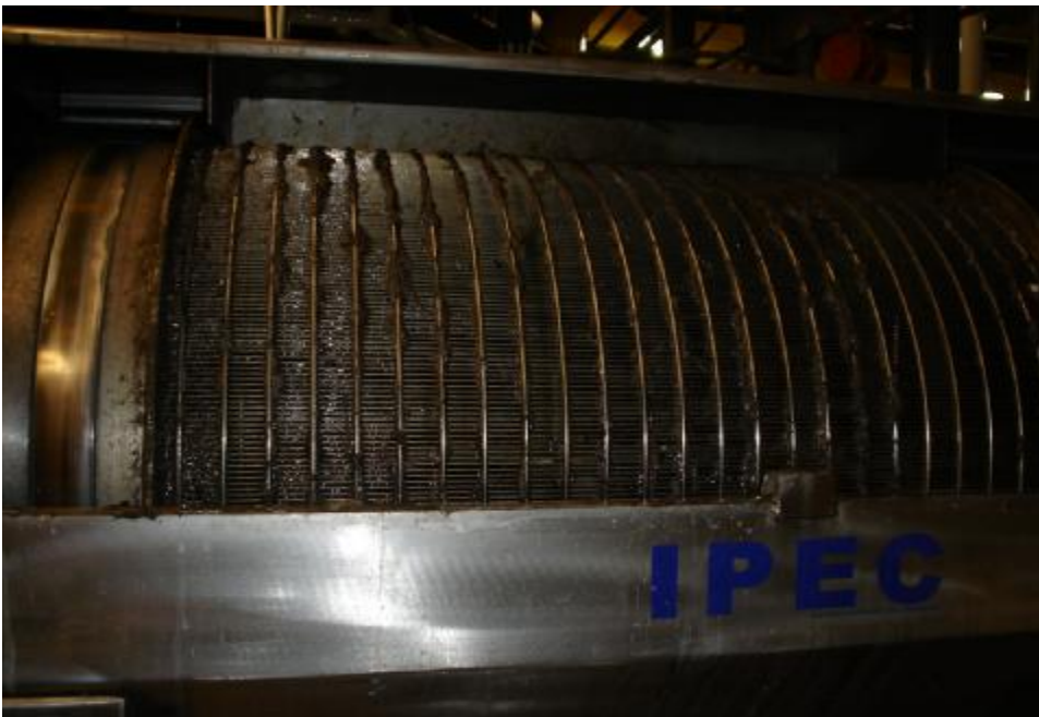
Photo 6. IPEC 30" x 36" with 3 mm rotary screen and ½ hp motor.
