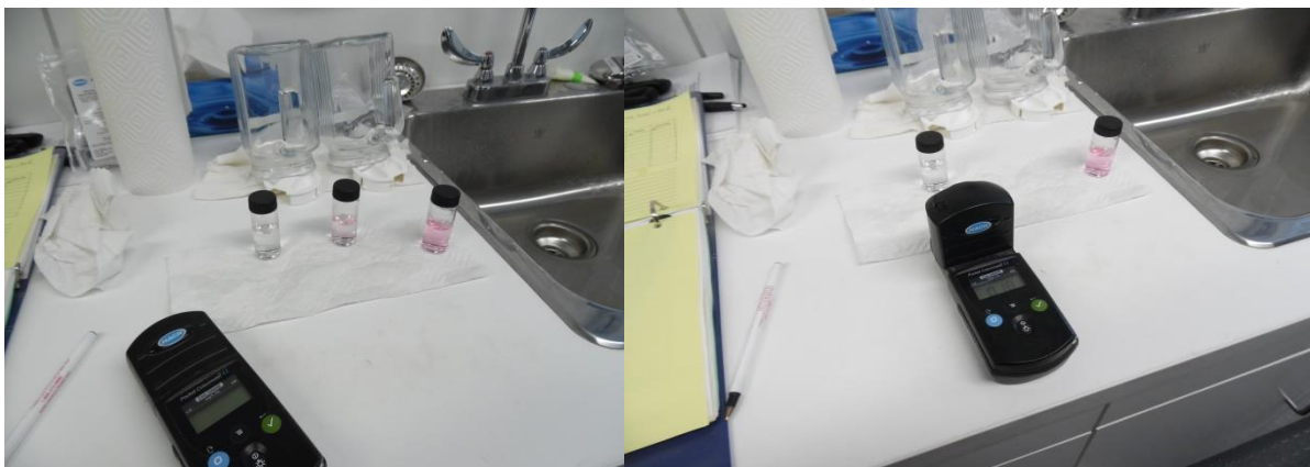
Free Chlorine sows 0.10 mg/l and 0.18 mg/l for samples from Truck#2 and truck #1
