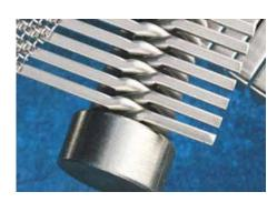
Looped wire profile screens are used in a variety of applications. Loop construction eliminates a welding requirement to join the rod and wire, as well as greatly increasing the durability of the screen in many applications.
