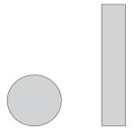
Johnson Screens round rods are available in diameters ranging from 0.125 in. (3.175 mm) to 0.500 in. (12.7 mm). Strip rods are available in widths from 0.070 in. (1.778 mm) to 0.188 in. (4.775 mm) and heights ranging from 0.375 in. (9.525 mm) to 2.0 in. (50.8 mm).
