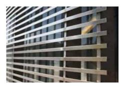
Johnson Screens standard welded construction uses resistance-welding in a continuous rolled motion to join the wire and rods. The resistance welds the continuous length of wire to the rods as it circulates.
