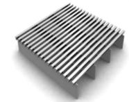
Johnson Screens shaped support rods range in widths from 0.029 in. (0.737 mm) to 0.151 in. (3.835 mm) and heights ranging from 0.102 in. (2.591 mm) to 0.120 in. (3.048 mm).
