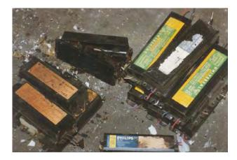
When substantial numbers of non-PCB ballasts are removed for disposal as PCB waste, this can add several hundreds and even thousands of extra dollars to the disposal cost. It is therefore important to ensure that all contractors are well experience in ballast identification.
