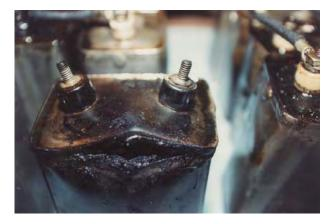
The high-level PCB liquid was released into the switchgear and the cable trench below. The staining was significant even though the actual volume of liquid was relatively small.
