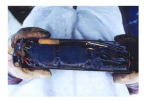
When the ASM is removed, the capacitor and copper coils are revealed.
