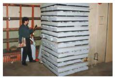
Prior to sorting, sometimes ballasts are stored on shelving units. This is OK if the ballasts are not leaking, if there are not too many of them and if the sorting is done expeditiously.
