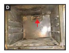
If you have determined that the gas oven capillary tubes and bulbs are mercury containing, the following procedure can be used to identify and remove the mercury gas safety valve control assembly.
