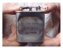
It is therefore important to keep in mind that when ballasts are involved in a fire, the contents of the capacitors inside the ballasts may rupture and release their contents into the zone of combustion.
