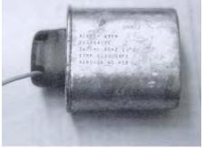
The capacitor contains approximately 17 ml (1.3 oz) of liquid PCBs with approximately half of this fluid absorbed by several layers of paper inside the capacitor. The risk of PCB leakage is quite low due to the construction of the capacitor.
