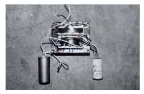
Although the capacitor is the component that contains PCBs, the ASM has been found to be PCB-contaminated in some cases to several thousand ppm (mg/kg) either from the manufacturing process or from a leaking capacitor.
