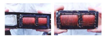
The value in the ballast is obviously the copper coils which are recovered and sent away for recycling.
