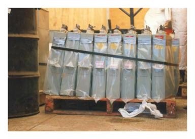
This technique will allow for the removal of more capacitors at one time, facilitate the use of a fork truck for moving loads and will permit efficient use of space in storage containers and on trucks when the capacitors are removed from site for disposal.
