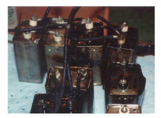
The pressure build up in the capacitors caused 5 of eight of the capacitors to explode and release their PCB contents.
