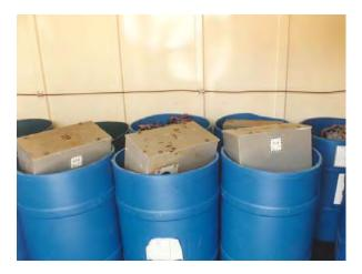
Leaking capacitors should be stored in proper open-top drums with lid, ring and secure bolt.
