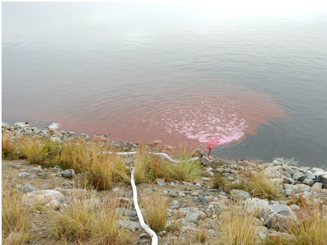
Photograph 14 – Dye plume diffusing north and east through lagoon after initial release
