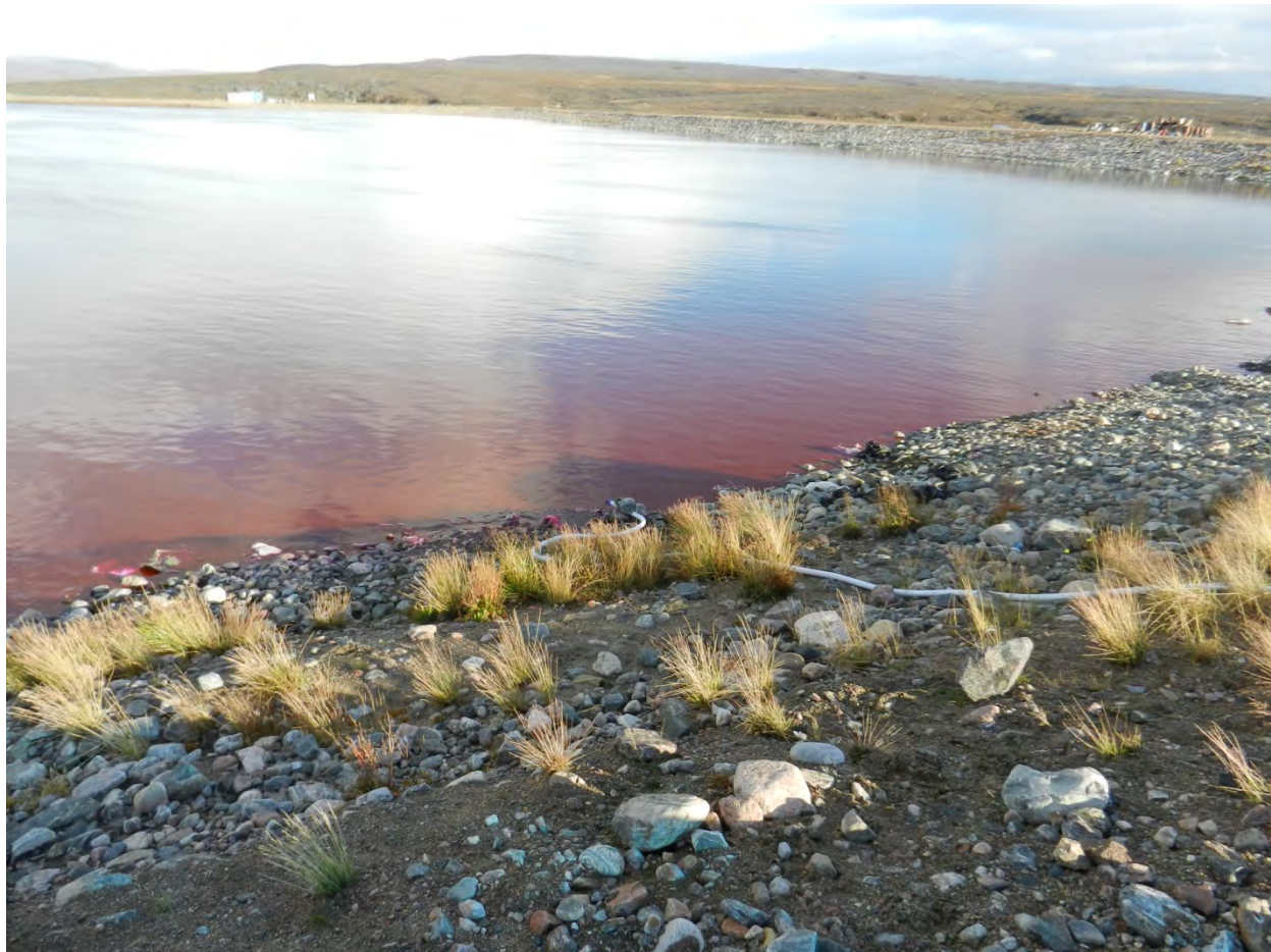
Photograph 16 – Progression of dye diffusion at release point approximately 1.5 hours after release
