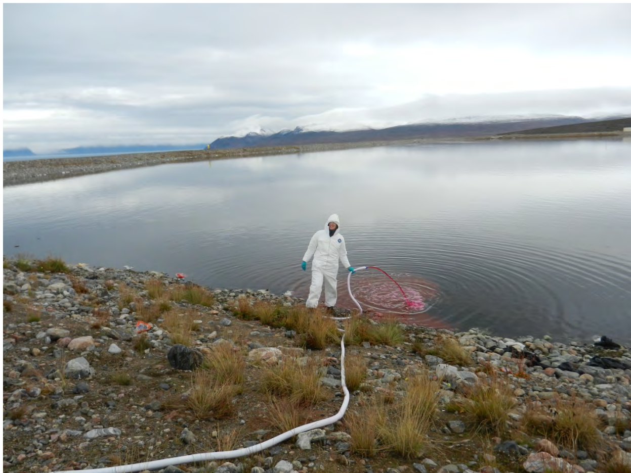
Photograph 13 – Mixed dye released into lagoon via gravity fed hose
