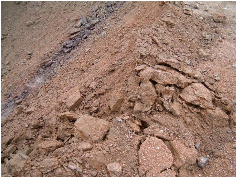
Photo 2 Close up of broken bedrock float weathering to sand and gravel at the quarry site.
