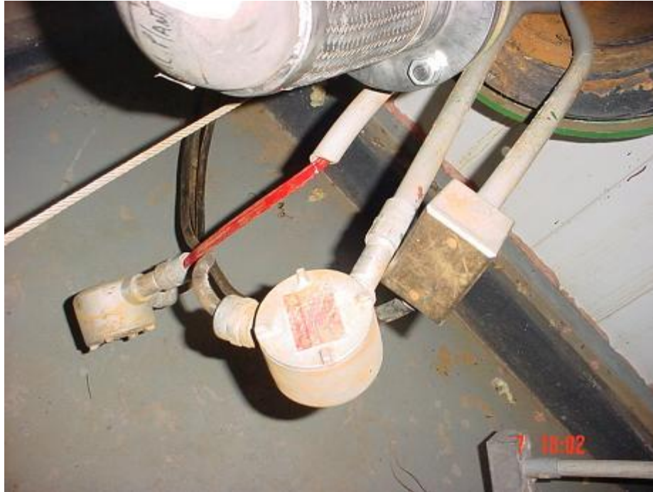
Figure E-11: Broken PVC Fittings
