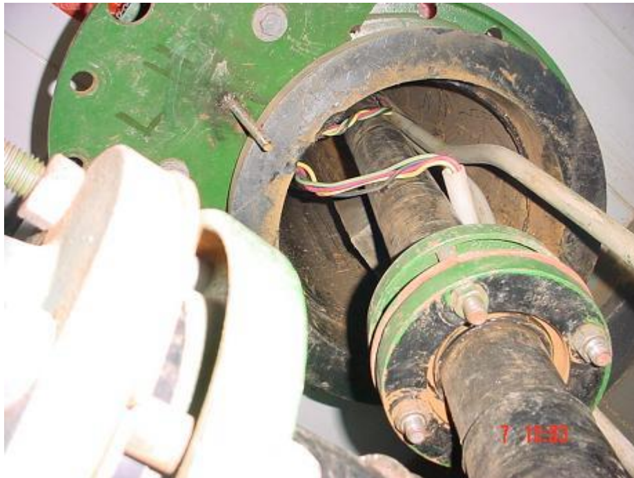
Figure E-12: Unprotected Conductors
