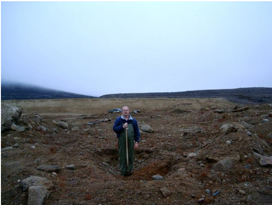
Photo 12 Bull dozed surface and test pits west of the water reservoir. Approximately 2.0 m of overburden to permafrost.
