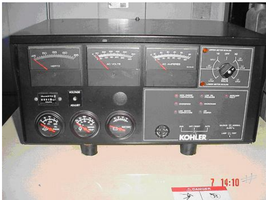
Figure E-2: Generator Control/Indication Panel
