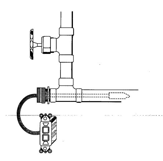
Submersible Heat Trace Freeze Protection System
