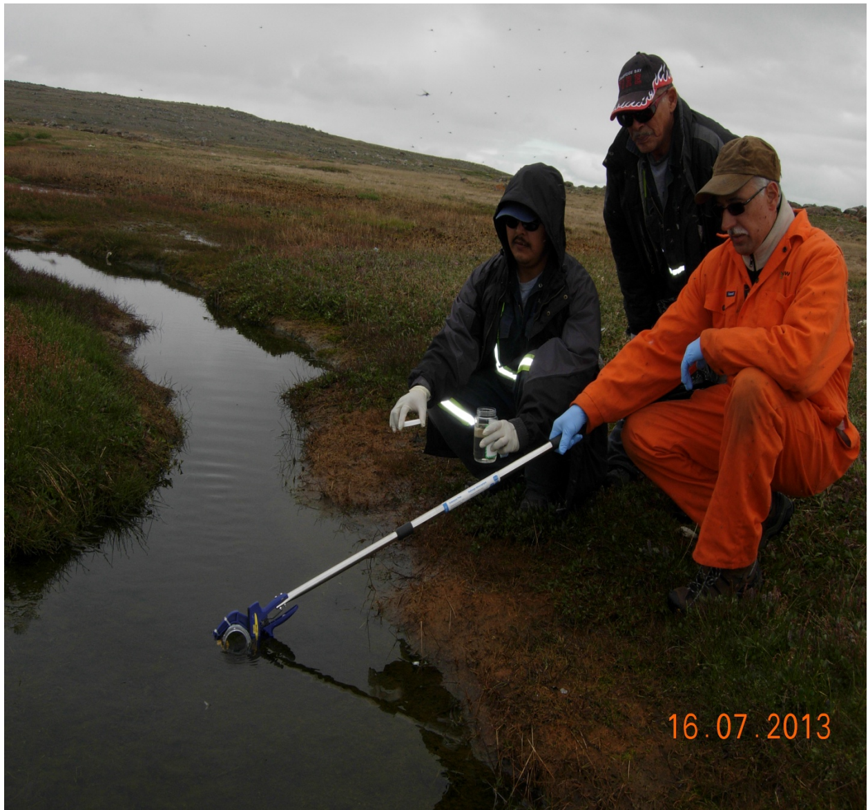
Picture 3: Shallow channel on wetland for effluent flow onto Ocean- sampling at the Final Discharge point for effluent test
