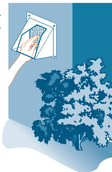
FIGURE 6 Checking exterior inlets and outlets
