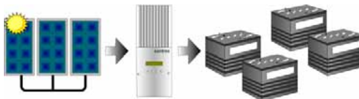
Figure 1-3 PV Charge Controller
