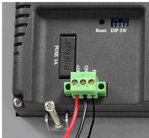
Typical Power Wiring
